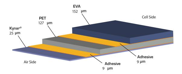
FLEXcon's multiGUARD® brand, a range of backsheets for photovoltaic modules, stands for multiple guarding properties – engineered to protect against moisture and humidity and provide superior partial discharge and high voltage insulation for proper functioning of the module. FLEXcon's line of backsheet products are designed to meet stringent industry standards and regulations.
