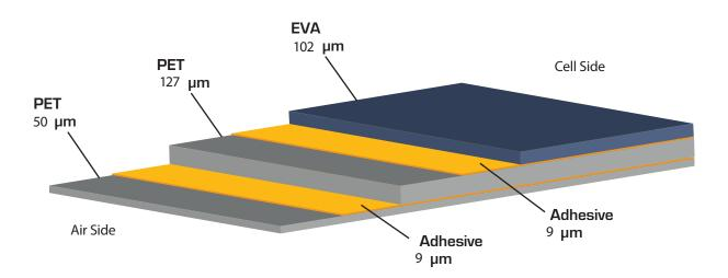
FLEXcon's multiGUARD<sup>\*</sup> brand, a range of backsheets for photovoltaic modules, stands for multiple guarding properties – engineered to protect against moisture and humidity and provide superior partial discharge and high voltage insulation for proper functioning of the module. FLEXcon's line of backsheet products are designed to meet required standards and regulations.
