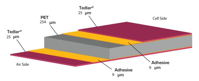
FLEXcon's multiGUARD<sup>®</sup> brand, a range of backsheets for photovoltaic modules, stands for multiple guarding properties – engineered to protect against moisture and humidity and provide superior partial discharge and high voltage insulation for proper functioning of the module. FLEXcon's line of backsheet products are designed to meet required standards and regulations.
