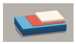
AKALIGHT ECS® 055 incorporates two basic layers with different functional importance. EPILAM and **CORLAM** carrying mainly the electrical and mechanical properties of the structure and bonding to the polymers used as pottings, sealants or adhesives, are combined into one layer. SUBLAM on the cell side provides a high bonding to the encapsulant.
