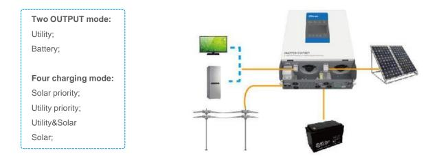
**Note:**When the battery voltage is lower than "Restore Auxiliary Module Charging Voltage( $V_{AON}$ )", the utility starts charging. When the battery voltage reaches to "Stop Auxiliary Module Charging Voltage ( $V_{AOF}$ )", the utility stops charging.
