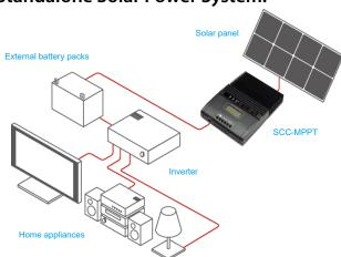
Combined MPPT technology and DSP controller, SCC-MPPT will convert best voltage to charge battery based on various temperature. Compared to traditional solar charge controllers, it allows your solar panels to operate at their optimum power output voltage, providing higher exciency up to 98% with lower power loss.
