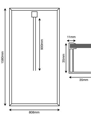
**Frame** Built-in aluminium angle m a k e s t h e f r a m e stronger and reliable on long-term. Angle is set inside the frame cavity.
