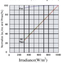
Note: the specifications are obtained under the Standard Test Conditions (STCs):  $1000 \text{w/m}^2$  solar irradiance, 1.5 Air Mass, and cell temperature of  $25^{\circ}\text{C}$ .
