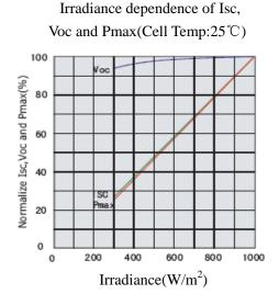
Note: the specifications are obtained under the Standard Test Conditions (STCs):  $1000 \text{w/m}^2$  solar irradiance, 1.5 Air Mass, and cell temperature of  $25\,^{\circ}\text{C}$ .
