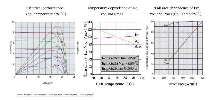
Note: the specifications are obtained under the Standard Test Conditions (STCs):  $1000 \text{w/m}^2$  solar irradiance, 1.5 Air Mass, and cell temperature of  $25^{\circ}\text{C}$ .
