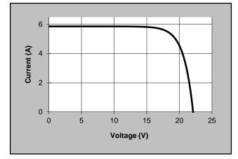
The electrical specifications are under test conditions of irradiance of 1 kW/m2, Spectrum of 1.5 air mass and cell temperature of  $25^{\circ}$ C. Minimum Power Output = Nominal Power - 10 %
