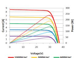
200W/m<sup>2</sup> Reference Data for 250W model. Cell Temp. 25°c
