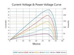
Excellent performance under weak light conditions: at an irradiation intensity of 200 W/m² (AM 1.5,25°C),95.5% or higher of the STC efficiency (1000 W/m²) is achieved
