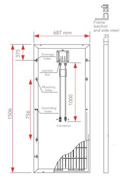
Module dimensions are expressed in mm with tolerance  $\pm 2$  mm ( $\pm 0.079$  ")
