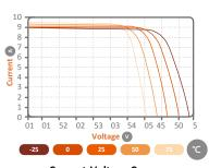
**Current-Voltage Curves** at Different Temperatures
