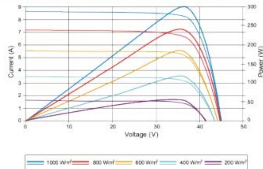
Excellent performance under weak light conditions: at an irradiance intensity of 200<sup>3</sup>W/m (AM 1.5, 25 °C), 95.5% or higher of the STC efficiency (1000 W/m<sup>2</sup>) is achieved
