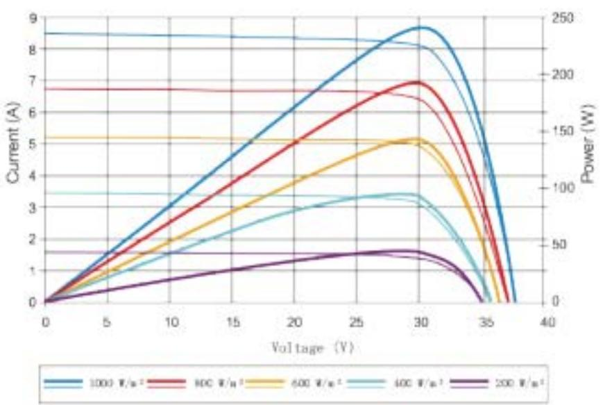
Excellent performance under weak light conditions: at an irradiance intensity of 200<sup>0</sup>W/m<sup>2</sup> (AM 1.5, 25 °C), 95.5% or higher of the STC efficiency (1000 W/m<sup>2</sup>) is achieved
