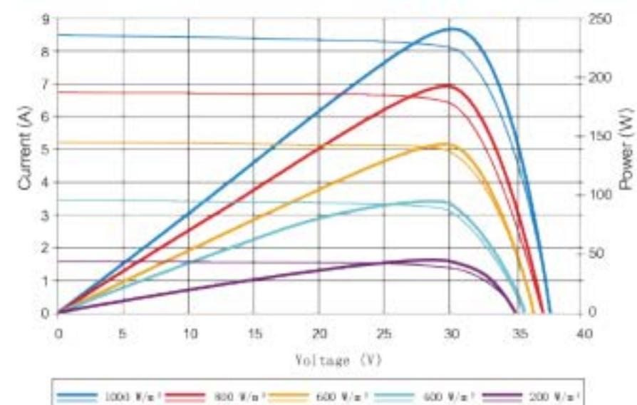
Excellent performance under weak light conditions: at an irradiation intensity of 200 W/m<sup>2</sup> (AM 1.5, 25 °C), 95.5% or higher of the STC efficiency (1000 W/m<sup>2</sup>) is achieved.
