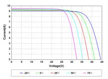
Current-Voltage Curves at Different Temperatures
