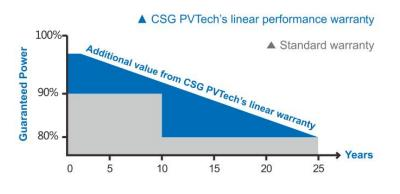
Warranty: For a period of 25 years commencing on the warranty start date, loss of power output of the nominal power output measured at STC for the products shall not exceed:
