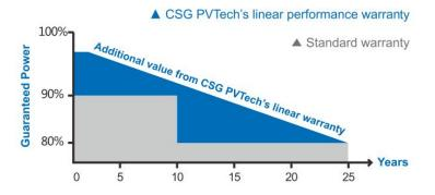
Warranty: For a period of 25 years commencing on the warranty start date, loss of power output of the nominal power output measured at STC for the products shall not exceed:
