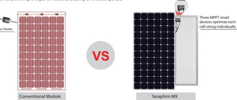
Under any condition, the Seraphim MX can optimize power output to enhance energy harvest. However, conventional modules or panel optimizer product will bypass cell-strings When they underperform. So seraphim MX will give higher energy prodution, eliminate hot-spots issues.
