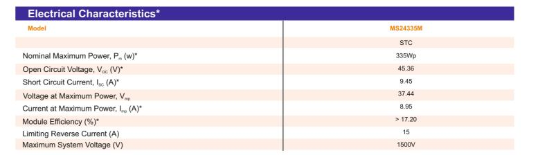
Standard Test Conditions (STC) : 1000 W/m2 irradiance, AM 1.5 spectrum and 25 Deg. C cell temperature
