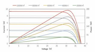
Excellent performance at 200W/m^2(AM 1.5, 25 C°): the conversion efficiency could be 96.2%
