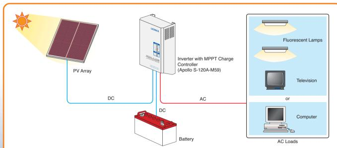
Solar home system is a stand-alone solar power system, uses for rural electrificatioin in remote areas where the utility grid is not available. The system consists of charge controller and inverter in the same enclosure. The charge controller controls charging current from solar array to storage battery and the inverter converts DC from battery to AC to supply to AC appliances. And built-in MPPT (Maximum Power Point Tracking) to maximize power generated by PV array.
