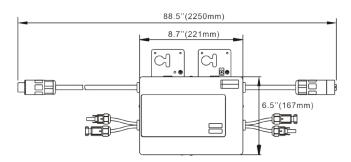
Our flagship product, the APsystems YC500A is a grid-tied microinverter with intelligent networking and monitoring systems to ensure maximum efficiency. Highly dependable and cost effective, the YC500A handles up to 310W modules with negligible clipping, delivering 250W AC per module with dual MPPT. Half the inverters and half the installation means real cost savings for residential and commercial customers.
