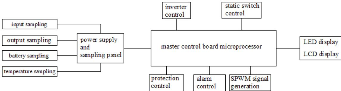
In addition to the above picture, other parts of inverter are including: inverter transformer, IGBT, silicon controlled, switch and etc.
