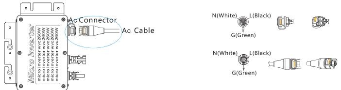
Step4 Plug the AC output line to main AC cable;
