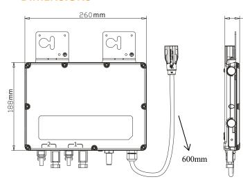
Our flagship new range of Grid-tied microinverters with Reactive Power Control (RPC) features includes the new YC600. The APsystems YC600 is a grid-tied microinverter with intelligent networking and advanced monitoring systems to ensure maximum efficiency. High efficiency, high reliability of the YC600 with 2 independent MPPT inputs, Maximum AC output power reaching 548VA. Half the inverters and half the installation means real cost savings for residential and commercial customers.
