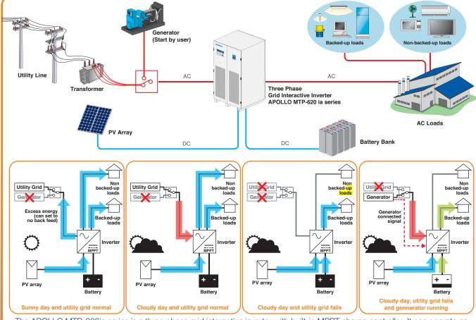
The APOLLO MTP-620ia series is a three phase grid interactive inverter with built-in MPPT charge controller. It can operate as grid tie inverter when utility line is available to reduce energy consumption. The inverter has two outputs. The output that provide backup power from storage and PV for the selected section house when utility line is not available and the output without back up power to help utilize PV power to reduce or prevent back feed power to
