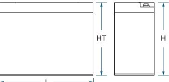
Tolerances are +/- 0.04 in. (+/- 1mm) and +/- 0.08 in. (+/- 2mm) for height dimensions. All data subject to change without notice.
