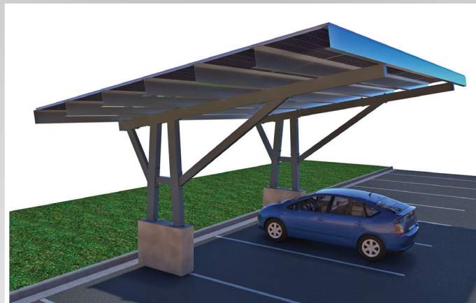
Mono-slope, South Foundation, 1 stall deep
