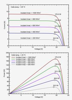
STC: Irradiance 1000W/m<sup>2</sup>,Module temperature 25°C,AM1.5 spectrum.
