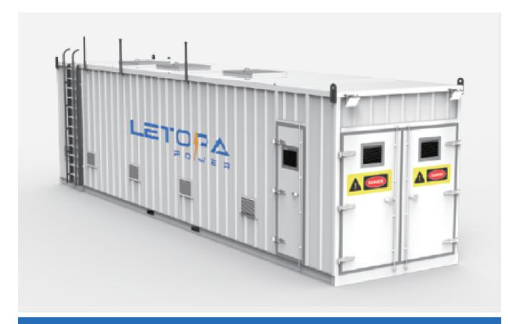
EnerContainer containerized high-voltage energy storage system, which can be connected to PV panels for solar charging. It can store over 500KWh of energy, which can meet the needs of most power supply (commercial, community, industria, etc). Built-in liquid heat thermal system ensures stable operation of battery modules under high&low temperature environment. Integrated energy storage converter, plug and play. Waterproof level meets IP54, can be installed outdoor.
