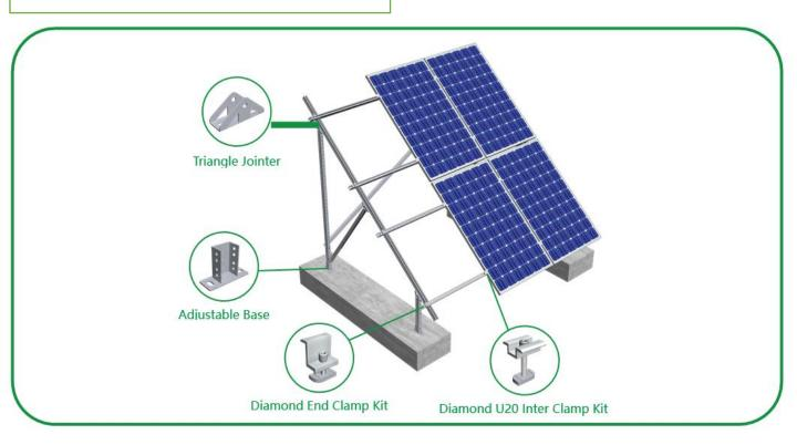
SRac Ground Terrace GT1 is suitable for large-scale and utility-scale solar PV power plant. Main components are made of hot-dip galvanized steel, with good performance of structure strength, stability and anti-corrosion, compatible with varied solar modules. Patented and certified system design ensure projects safety and quick installation.
