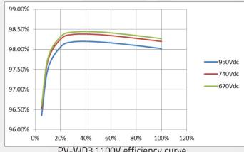
PV-WD3 1100V efficiency curve
