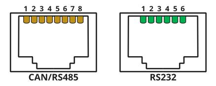
Figure 4 - CAN/RS485 and RS232 connections
