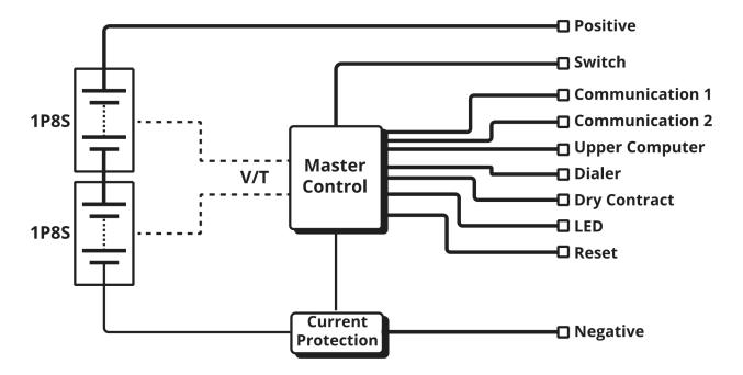
Figure 1 - System schematics
