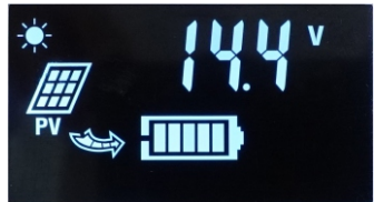
6. Floating charge voltage setting
