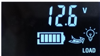
7: Discharge recovery voltage setting
