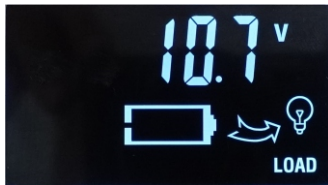
8: Discharge cut-off voltage setting
