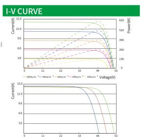
\_\_ 25°C \_\_ 50°C \_\_ 75°C Voltage(V)
