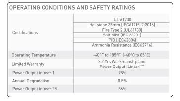
NOTE: Values at standard test conditions[STC: air mass AM1.5 irradiance 1000W/m2, temperature 25°C).
