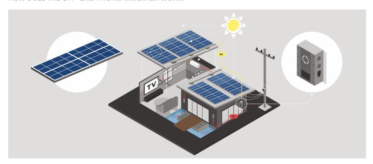
The efficiency of a solar PV system depends on the selection of the right inverter, or solar inverter. The inverter performs a key function in this system, changing the DC current generated by the solar PV panels into AC current used by household appliances.
