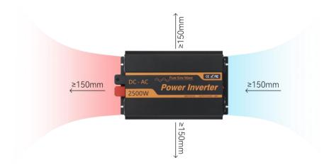
**Note:** Only suitable for installation on concrete or other non-combustible walls.
