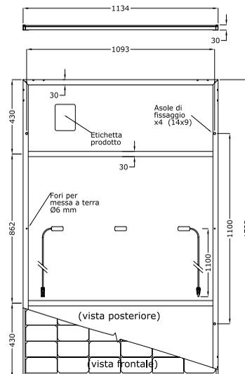
Note: dimensions in mm, tolerance +/- 2 mm
