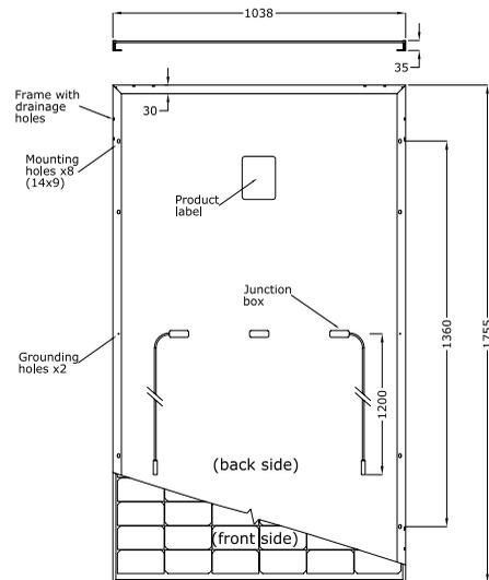
Note: dimensions in mm, tolerance +/- 2 mm
