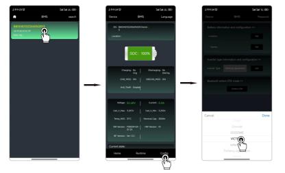
Step 2: Open the SUNESS app, search the device serial number and tap to choose it.Step 3: Tap the Configure and select the inverter type
