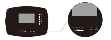
The BMS features 6 external LED indicator lights. 1. 4 white-green capacity indicator lights. 2. 1 red alarm indicator light. 3. 1 withe-green operational indicator
