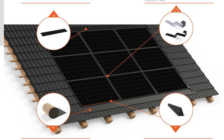
The foil is a highly robust and weather resistant self-adhesive foil which is used to seamlessly drain roof water from the PV modules to the bottom of the PV array. The foil is not required on PV arrays that reach to the bottom of the roof as the roof water is guided directly into the gutter.
