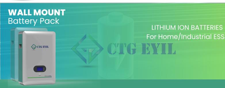
This CTG Wall Mount battery pack is applicable for residential and commercial energy storage system, which is assembled with 3.2V 104Ah lithium iron phosphate cell in 2P8Sconfiguration, and intelligent BMS form 25.6V200Ah lithium battery system.
