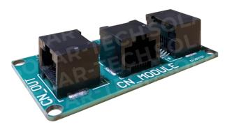
The MDC module acts as an intermediary when your inverter communicates with the batteries via the CAN port.
