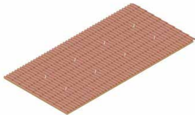
Step 3: Mount all the hooks with spacing as specified in the drawing with good alignment
