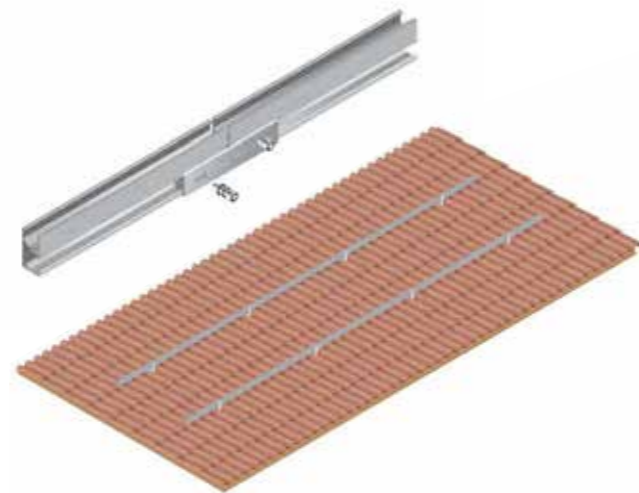
Step 4: Secure the rail on the hooks
