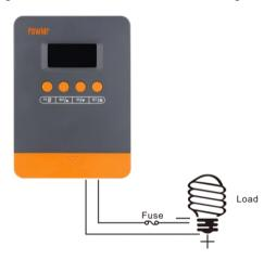
**Step 5.Pre-start check:** Refer to the wiring diagram below. If all connections are accurate and secure, close the battery and PV array breakers in sequence.
